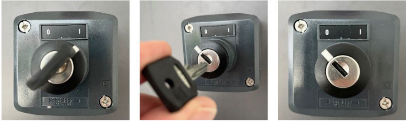
Figure 22: Sequence for reactivation of key switch
